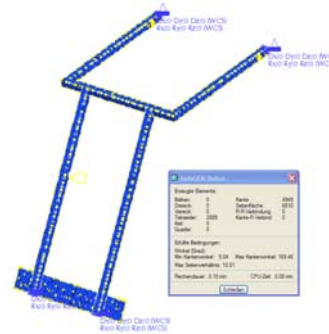
Fig. 8 – Mesh 3D model of the optimized version
