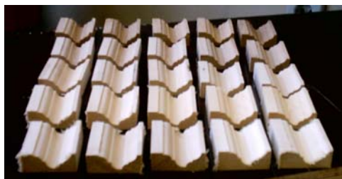
Fig. 1. Test samples for measuring the roughness
