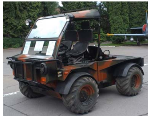
Fig. 2.1 The light off-road articulated vehicle DAC 2.65 FAEG
