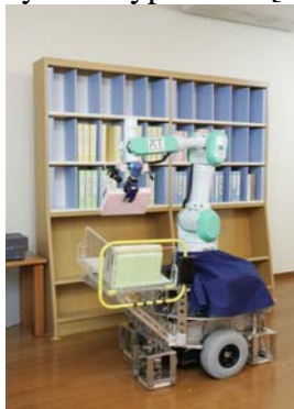
Fig. 4 The librarian robot system, the intelligent floor, and the intelligent bookshelf. (B. K. Kim et al., 2008)
