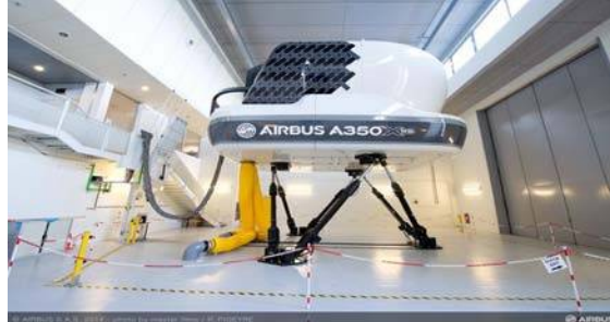
FIG.4.2 Full Flight simulator Source: www.airbus.com
