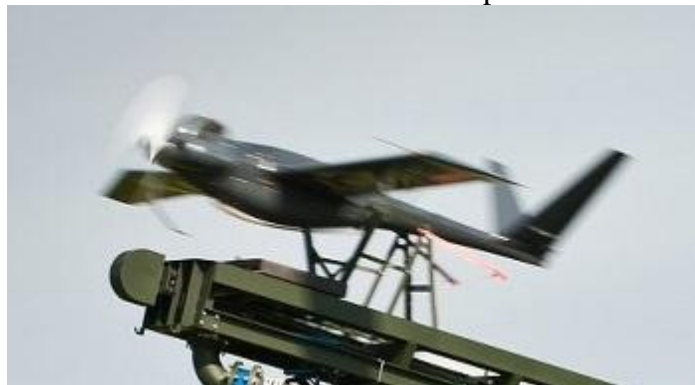
FIG. 1. Small UAV launch from an air-powered catapult.
