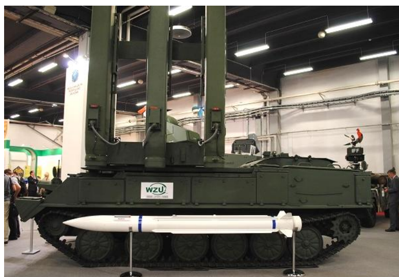
FIG. 3. The SA-6 have a certain up-grade potential - here the Polish variant w. RIM-162 ESSM
