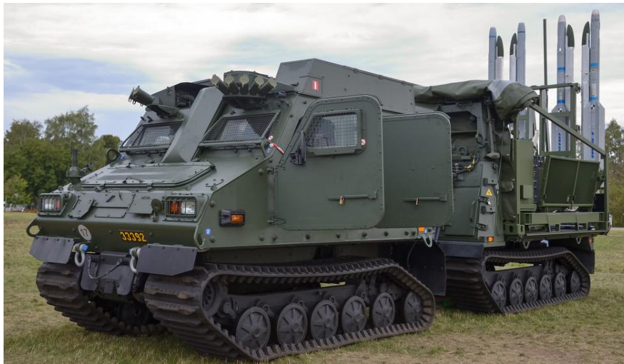
FIG. 4. IRIS-T AAM is directly used in SLS AD derivative -here the Swedish variant
