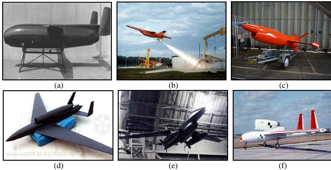
FIG. 2. Turbojet engine applications in UAVs , (a) Radioplane Q-1 [22], (b) Ryan Firebee [23], (c) Nord Aviation CT20 [24], (d) Teledyne Ryan AQM-91 Firefly [25], (e) Ryan Model 147 Lightning Bug [26], (f) Boeing YQM 94A Compass Cope [27]
