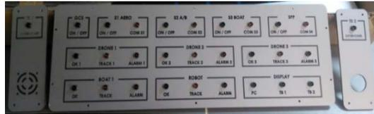
FIG. 3.4 Realization of the upper signaling panel through CNC technology
