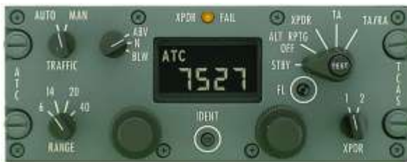
FIG. 2 The Mode S/TCAS control panel, [7]
