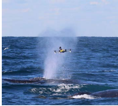
FIG. 2. UAV collecting a sample of whale blow [23]
