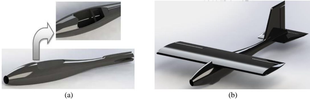
FIG. 3 RC aircraft design: (a) structure of the fuselage, (b) final model of the RC aircraft.
