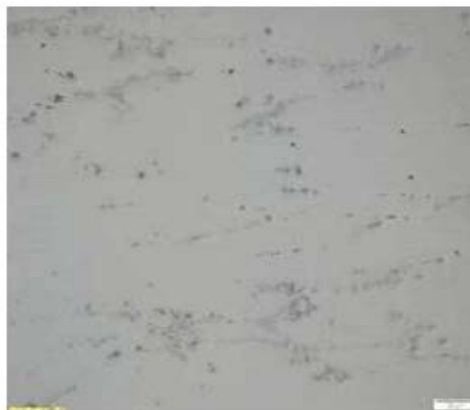
FIG. 5 The metallographic structure after quenching at 540 °C, 1 h/water and ageing at 177 °C for one hour. HF etching. 100X magnification.
