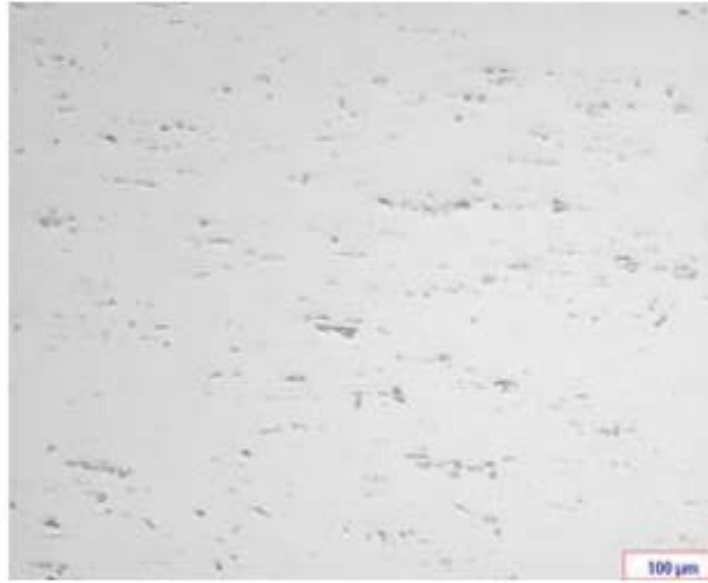
FIG. 3 Metallographic structure after quenching from 550 °C, holding for 30 minutes and cooling in water. HF etching. 100X magnification
