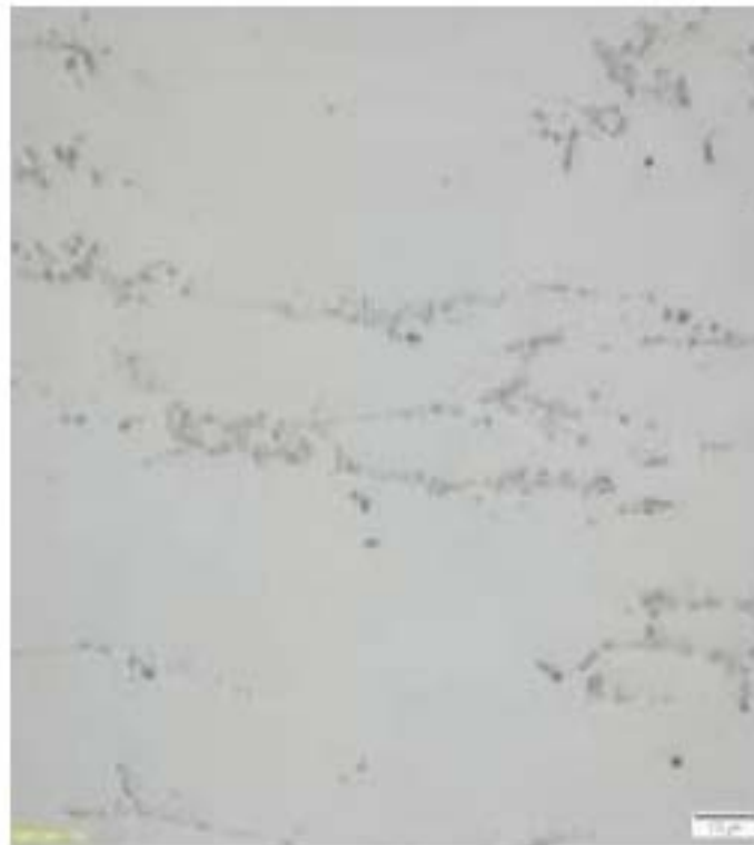
FIG. 4 Metallographic structure after quenching at 540 °C, 30 minutes/water and ageing at 177 °C for 30 minutes HF etching. 100X magnification
