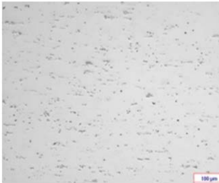
FIG. 2 Metallographic structure after quenching from 540 °C, holding for 30 minutes, cooling in water. HF etching. 100X magnification
