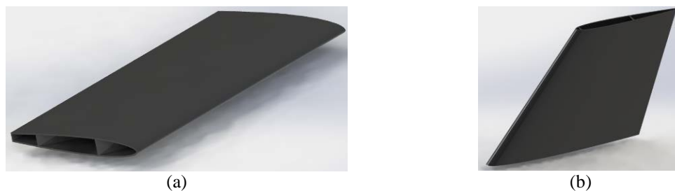
FIG. 2 Three-dimensional model: (a) horizontal empennage, (b) vertical empennage.
