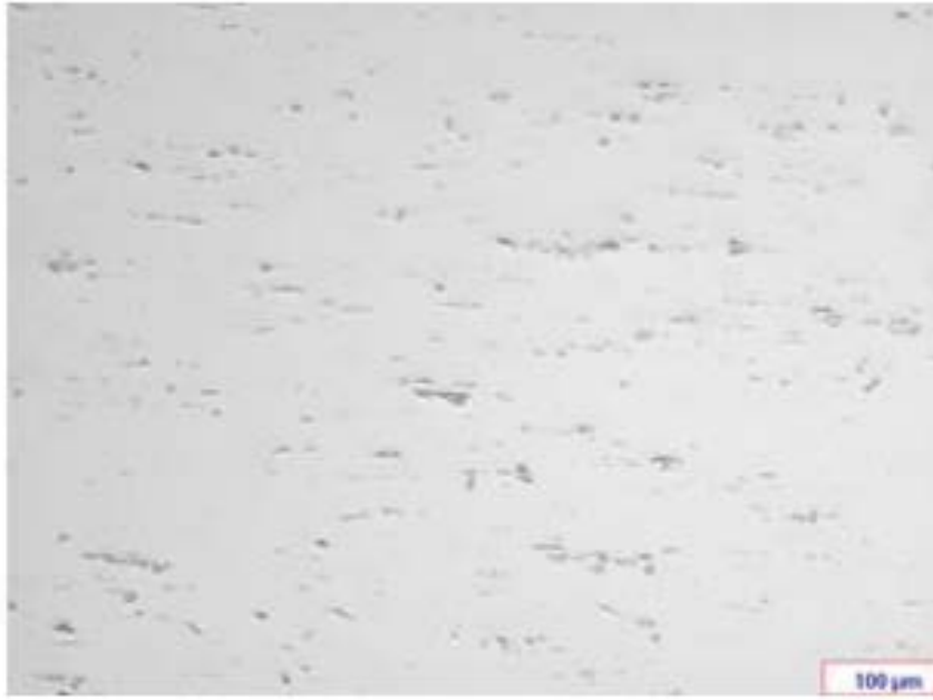
FIG. 1 Metallographic structure after annealing (in the initial state). HF etching. 100X magnification
