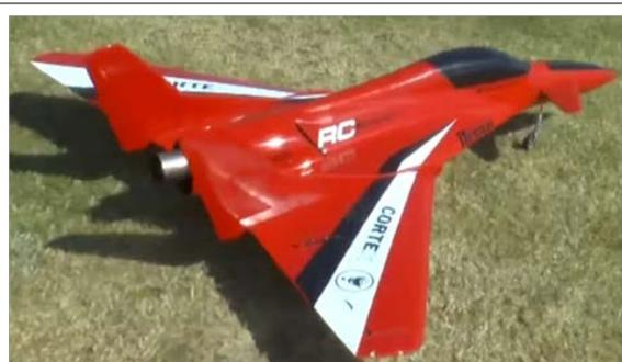
**FIG. 2** Corte UAV, canard configuration with vectored thrust
