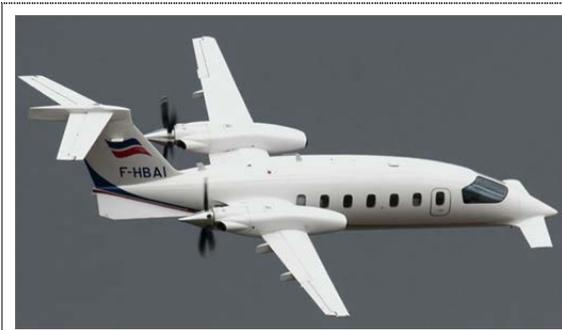
**FIG. 1** Piaggio P 180 Avanti with two horizontal empennages
