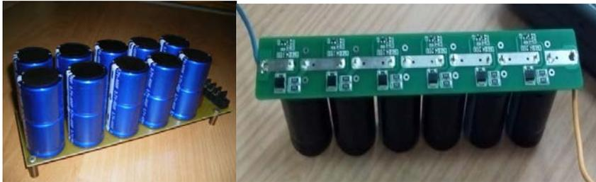
FIG. 3. Super Capacitor Batteries (Heter, left,  $U_{max} = 13.5$  V; GreenCap, right,  $U_{max} = 16.2$  V)
