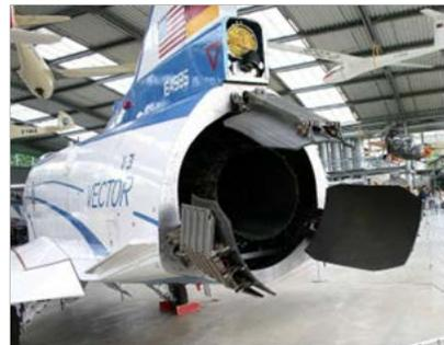
**FIG. 4** Vectored thrust obtained with deflection shutter
