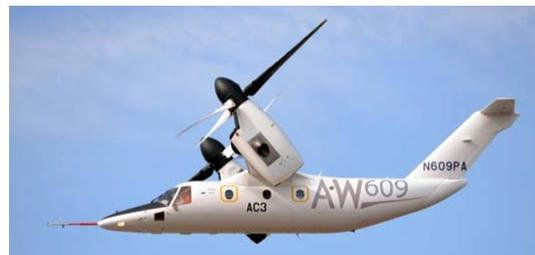
**FIG. 6** Tilt rotor vectored thrust
