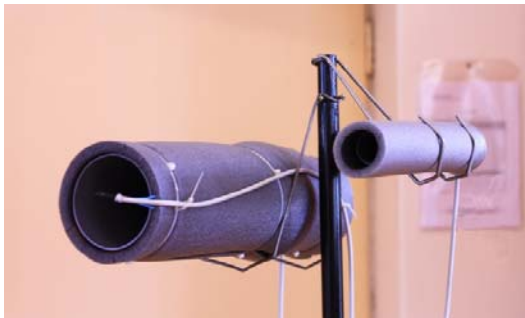
Pic. 4.1. RX (MIC – the smaller tube) and TX (Speaker – the bigger tube).
