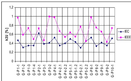
Fig. 5. Voltage unbalance negative factor K2U for the issues from „PT-X”
