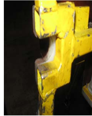
Fig. 6 Details including plastic wear plates, due to friction welding electrodes.
