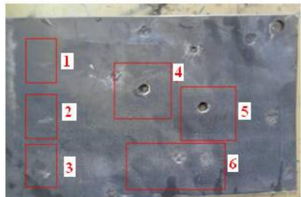
Fig. 4: Areas of hardness measurements on a sample
