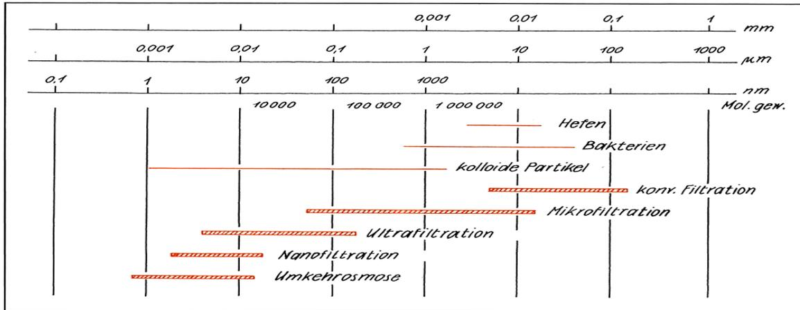
Fig. 2. Particle and filter pore size ranges
