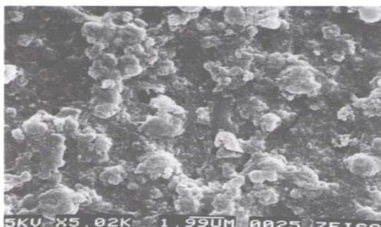
Fig.6. Particulate material deposited on the membrane surface
