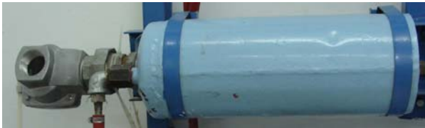
Figure 7. PID with metallic vessel
