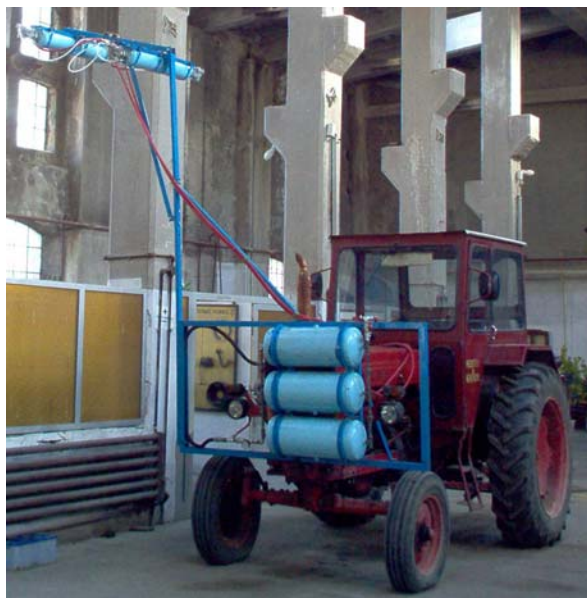
Figure 5. Modular Equipment for Nuts Harvesting by Pneumatic Impulses – MEHPI
