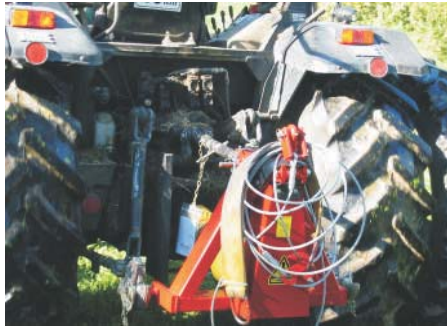
Figure 1. Mechanic rope shaker device
