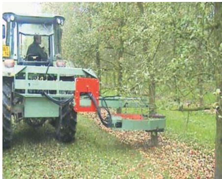
Figure 2. Hydraulic trunk shaker for half standard trees
