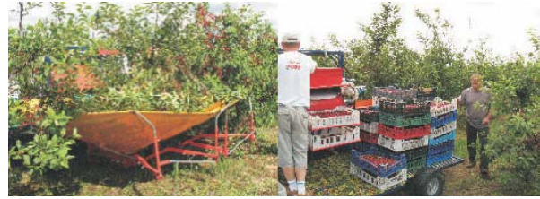
Figure 4. Umbrella harvester with shaker
