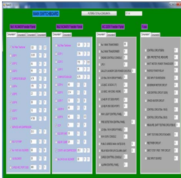
Figure 7. Main distribution panel for underway regime
