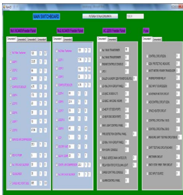
Figure 8. Main panel for loading / unloading regime
