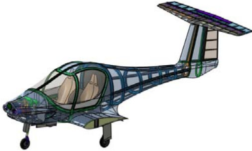
Fig. 9 CAD model of the fuselage
