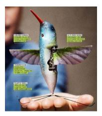
FIG. 2. Nano Air Vehicle "Hummingbird"
