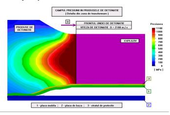
**FIG. 5.** Presure field in detonation products: D - the detonation wave front; 1- the movable plate; 2- the basic plate; 3- the protect layer.
