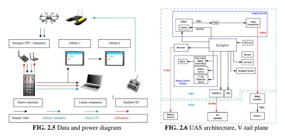
*Modules and connection diagram.* The UAS architecture contains the two functional entities: the air vector (UAV) and the ground control station (GCS).
