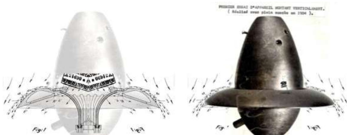
FIG.3 The Coanda Effect thruster successfully tested in 1932
