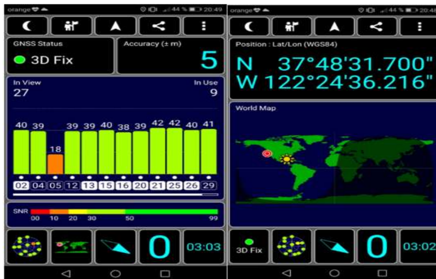
FIG.4 View of the fake data received by the GPS Test application
