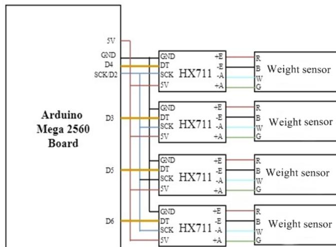
FIG. 4 Block diagram of the weight sensor
