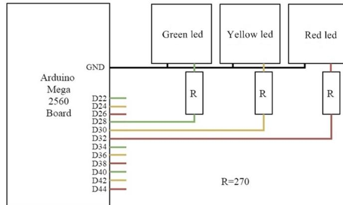
FIG. 8 Block diagram for LEDs
