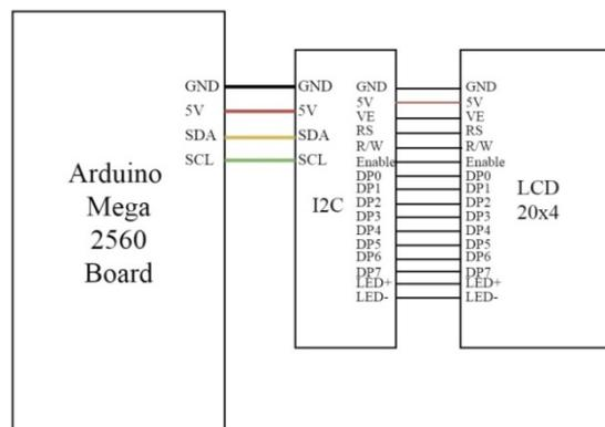
**FIG. 6** Block diagram for LCD
