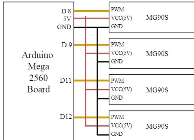
**FIG. 5** Block diagram of servo motors
