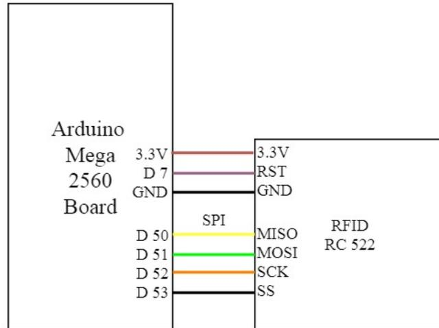
**FIG. 7** Block diagram for RFID
