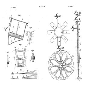
FIG. 13 Safety device for automatous parachute - Kotelnicoff Gleb - This invention consists of a safety device where the parachute is closed and at the moment of pulling up the parachute is thrown out [23]
