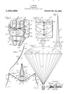
FIG. 11 Parachute – Smith Floyd - This invention provides a dependable means for causing the straightening out and opening of the parachute under all conditions, including certain conditions under which the present type of parachute is totally inoperative or deficient in operation [21]
