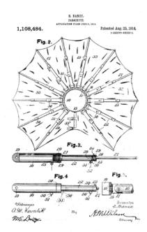
FIG. 10 Parachute – Stephan Banic - This invention relates to a parachute of collapsible type which may be easily and quickly attached to the body of the wearer and readily distended to operative position when desired [20]
