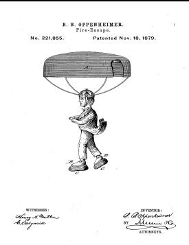
**FIG. 12** Improvement in fire-escape - Oppenheimer Benjamin - This invention consists of a parachute attached, in suitable manner, to the upper part of the body, in combination with overshoes having elastic bottom pads of suitable thick mess to take up the concussion with the ground. [22]
