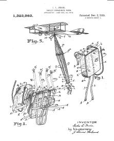
**FIG. 9** Safety parachute-pack – Leslie L. Irvin -This invention relates to safety parachute packs, particularly to that kind which includes the systematically packed parachute and connections in a neat sack. [19]
