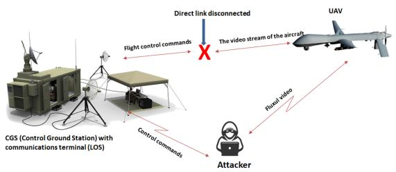
FIG. 4 MITM attack on a UAV [10]
