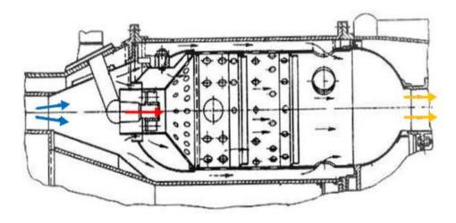
FIG. 2 The combustor. Mix gases circuit, [7].
