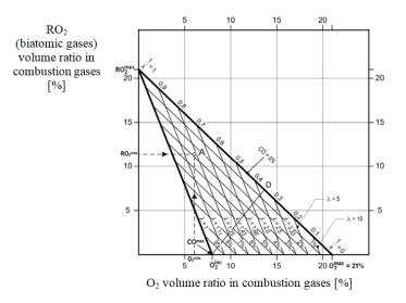
FIG. 1 Oswald diagram (combustion triangle), [2].
