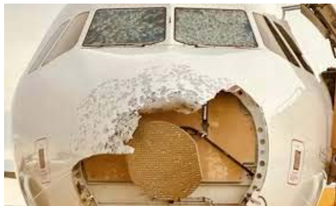
FIG. 3. Austrian Airlines Mayday after severe hail damage [5]
