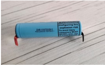
FIG. 10 Battery Pack (LG 3.7V, 3200 mAh)
