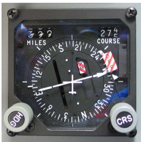
Fig. 3 Indicator HIS in L-159 aircraft
