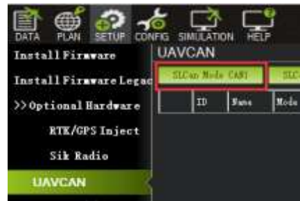
FIG. 11 Enabling CAN settings on Mission Planner software
