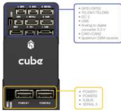
FIG. 19 Cube Top connectors [12]
