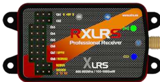
FIG. 18 RXLRS- radio control and data link receiver [10]
