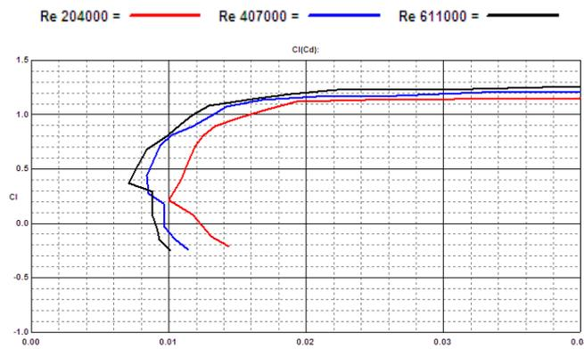
FIG. 3.4 Polar  $C_l$ - $C_d$  - Profili
